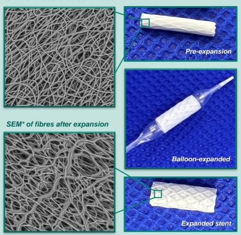
Elastic fibres show no breakages. Coating stayed intact with no delamination or tears.
